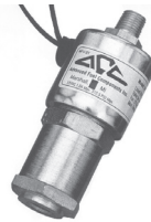
AFC-418B FILTER LOCK-OFF VALVE 1/4" FNPT Inlet and 1/4" MNPT Outlet 12 Volt Ceramic magnet traps fine metallic particles. High performance filtration capability with integrated 20 micron replaceable filter.
