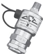
AFC-152 INLINE FILTER SHUT-OFF VALVE 1/4" FNPT Inlet 1/4" MNPT Outlet 12 Volt Replaceable filter
